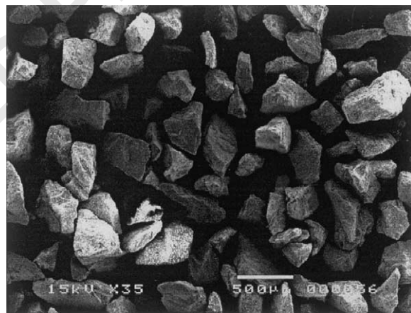
Fig. 1. Scanning electron microscopy (SEM) image of bovine HA particles sintered at 1100^\circ\text{C} . Particles present irregular shapes. Bar: 500 \mu\text{m} .
